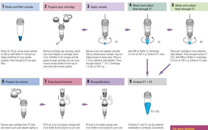
and attach Luer-Lock adapter tightly to top of cartridge.
